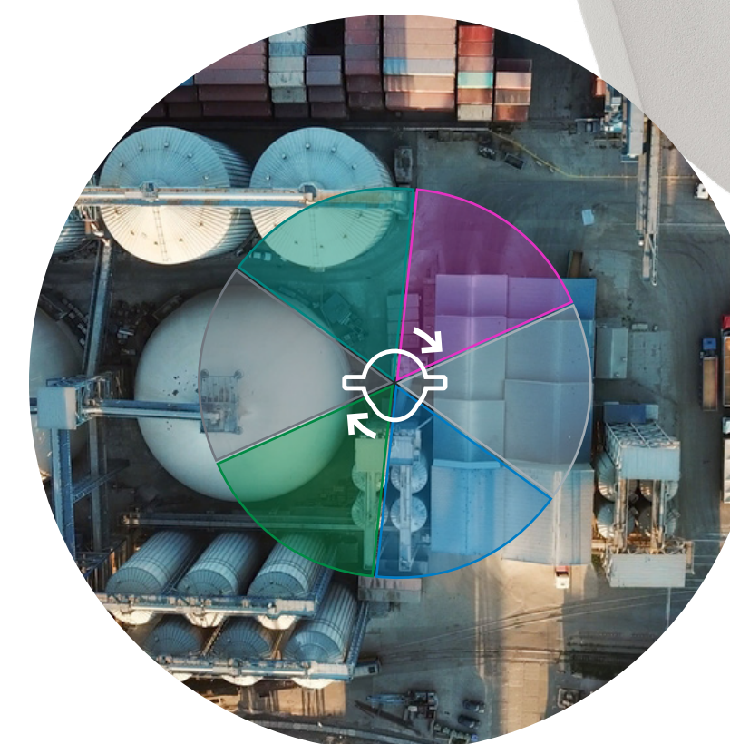
MIC IP fusion 9000i 9mm lens: six pre-positions for a 360 degree coverage of the full scene in less than 30 seconds
